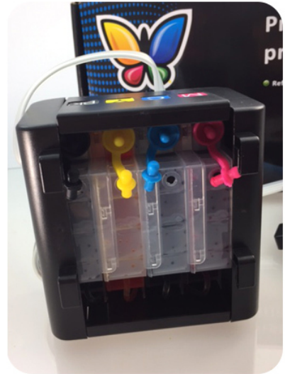
4. Remove all the coloured small plugs from the tank unit (leaving the larger plugs in place/closed).
