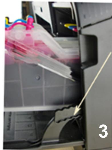
**3- Remove the small plugs and put the air filters on top of the small hole.**
